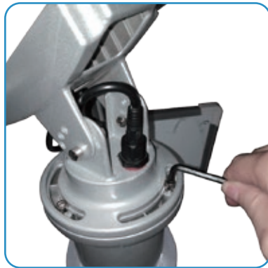
Step 4: Adjusting angle on the horizontal for 360°
